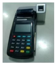
HHT FP is a time attendance system with inbuilt GPRS and WiFi modules, thermal printer along with inbuilt contactless card reader. This device comes with a fingerprint scanner as an external peripheral. The whole assembly is shown above.
